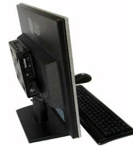
Linutop placed on the back of a flat panel, with the monitor mounting bracket accessory
